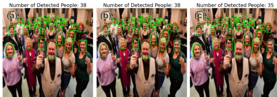
Figure 9. Sample of human detection results using fine-tuned YOLO11 in high-density conditions for (a) S1, (b) S2, and (c) S3 (source: validation dataset).
