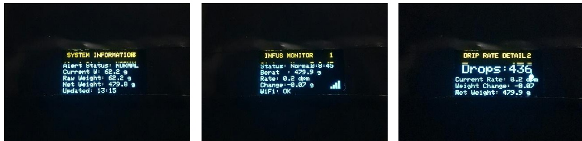
Fig. 8. OLED Display Interfaces: (a) Main Status. (b) Status & Alert. (c) Drip Statistics.
