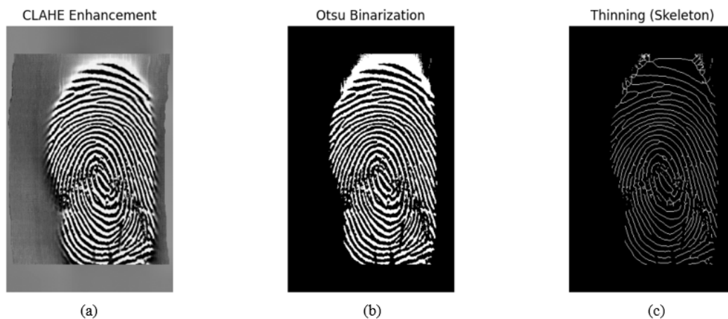
Figure 9. (a) Fingerprint Image after CLAHE Enhancement, (b) Fingerprint Image after Otsu Binarization, and (c) Fingerprint Image after Thinning (Skeletonization)
