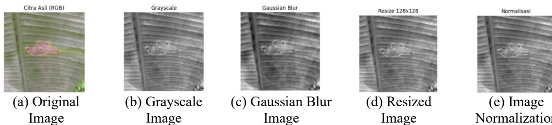
Figure 2. Image of Leaf Image Preprocessing Results (a) Original Image, (b) Grayscale Image, (c) Gaussian Blur Image, (d) Resized Image and (e) Image Normalized pixels to the range [-1,1]
