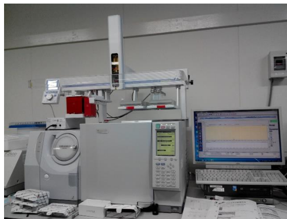
Fig. 1. The instrumen of GC-MS used to identify the hexylene glycol in perfumes
