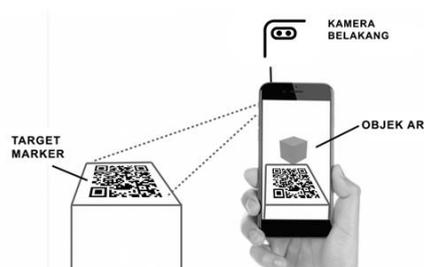
Gambar 2. Cara kerja marker based tracking
